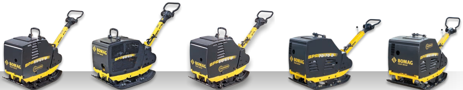
BPR 55/65 D Operating weight: 455 kg Centrifugal force: 55 kN Working width: 650 mm BPR 60/65 Operating weight: 400 kg Centrifugal force: 60 kN Working width: 650 mm BPR 60/65 D Operating weight: 460 kg Centrifugal force: 60 kN Working width: 650 mm BPR 70/70 D Operating weight: 580 kg Centrifugal force: 70 kN Working width: 700 mm BPR 100/80 D Operating weight: 710 kg Centrifugal force: 100 kN Working width: 800 mm
